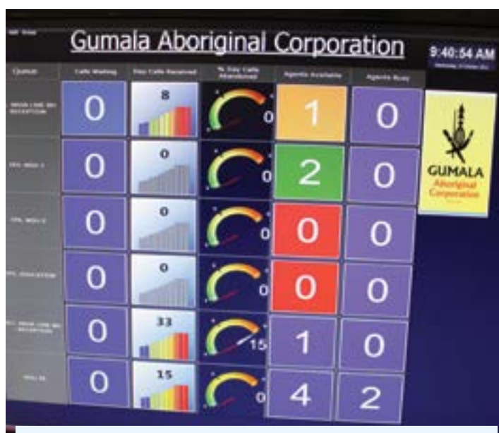
GAC's telephone network monitoring system, which monitors all phone calls and displays the information visually to allow the Reception and Member Services teams to view the live call information.
